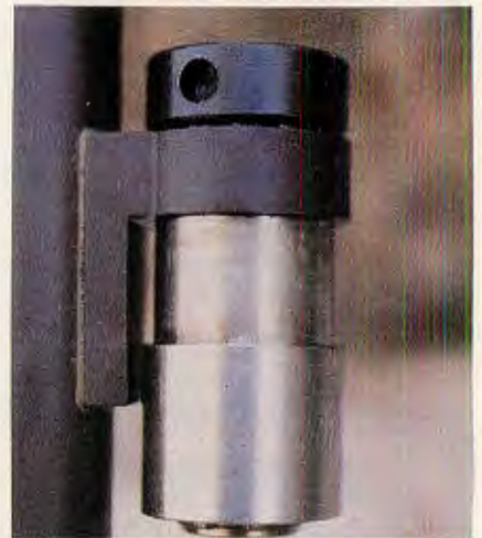
ABOVE: Gas system: stationary stainless-steel piston surrounded by sleeve which traps gas and moves rearward to strike against the slide extension tube.
